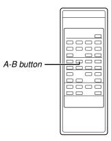
1 During playback, press the A-B button on the remote control unit at the point (A) where you want to start A-B repeat playback.
